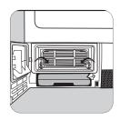
2. To pull out the condenser, first turn the two red stops downwards.
